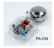
**Bell Electric 6 Volts, model PA-239,** twin coil, for battery or transformer operation. Operation on 6V DC, transparent moulded design with plated bell 50mm diameter, the coil sand terminals are enclosed under a snap-on-transparent moulded cover. Can be fixed to the wall, Dimension: 70mm x 135mm x 33mm high.,
