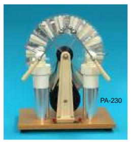
Winshurt Machine, Model PA-230, two plates are supported in two rigid uprights and driven by belt in opposite direction. Providing the positive and negative charges, and the high tension DC voltage used in the electrostatic experiments, with the discharge distance of 30-40mm,. Circular disc diameter: 270mm.
