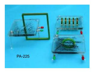
Magnetic Field Experiment, Model PA-225, 3 units (plates size: 105 x 95 x 8 mm approx.) for domonstrating the magnetic field produced by the DC current pass through the straight conducting wire, the ring conducting wire or the solenoid. Design for overhead projection, 4 - 6V DC required.
